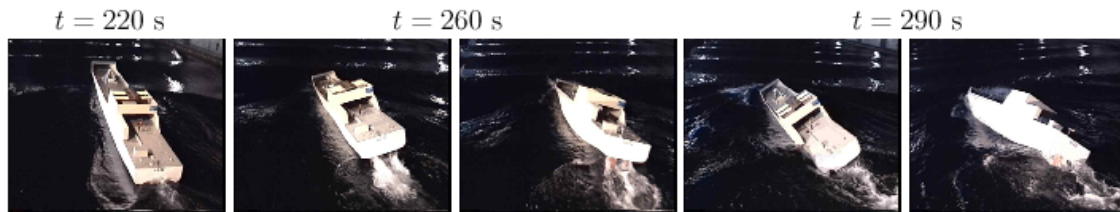
Figure 12: Parametric excitation of the RO-RO vessel (compare Fig. 10) — model scale 1:34.
